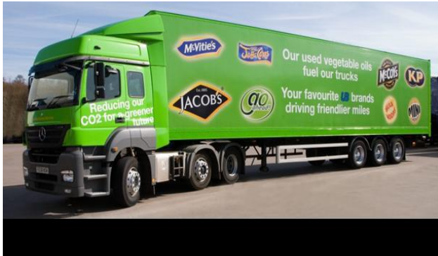
Duel fuel biodiesel Used Cooking Oil United Biscuits (Low Carbon Truck Trial)
